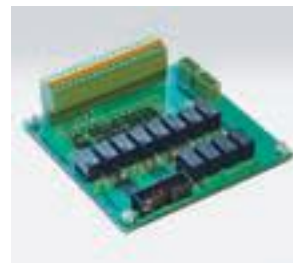
Alarm and Status Notification Board
